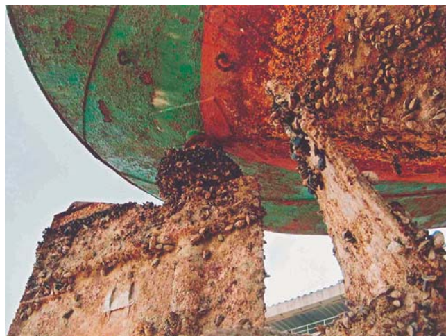
Slika 1 Obraštanje podvodnog dijela broskog trupa Figure 1 Fouling of the underwater part of the ship hull
