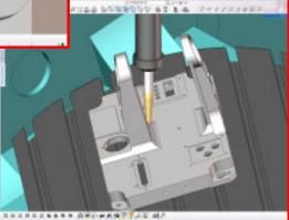
of the associated elements and generates the NC program. **The tool path is formed taking into account the predefined machine kinematics** for Multi-axis machines. Multi-axis machining comprises 2.5, 3 and 4 axis milling strategies. To carry out machining of the same part on a machine with a different configuration, all that is required is the selection of the new machine and subsequent recalculation of the operations.
